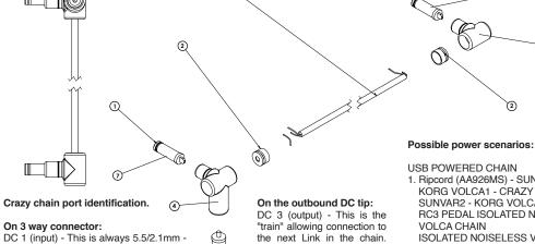
DC 1 (input) - This is always 5.5/2.1mm - allowing the "train" to be connected to Crazv Chain.
